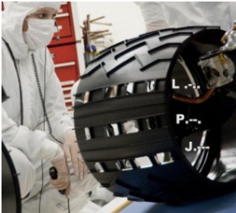
Detail of Mars Science Laboratory Curiosity Rover with tread pattern that will leave an impression on the Martian surface spelling "JPL" in Morse Code (---- ···· ····). Photo courtesy of NASA/JPL.
